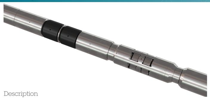
The Tubing Packer (TP) is a packer for hanging off heavy loads in the well. The loads are carried via the packer main mandrel and the setting tool mandrel into the running string. This is achieved without interfering with the setting compression forces required for the element sealing. Hence, the tested and well proven technology from our standard plug and packer program is applied.
